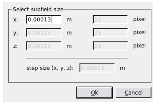
Figure 40 Subfield Features: dialog for specifying the subfield size.
