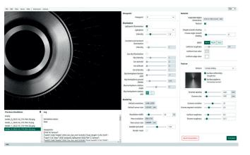
V-POI simulation editor showing the simulation of the blisk object when imaged from above using ring light illumination (see highlighted viewpoint on the previous page).
