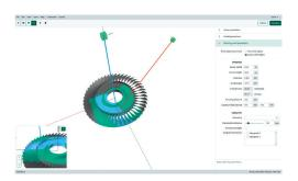
Above:V-POI uses a 3D model to simulate multilayered texture and defects on it, which are further used to generate an automatically annotated dataset.
