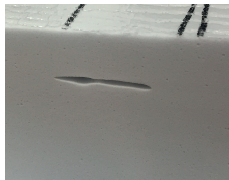
Foam with air inclusion: specimen (left) and 3D terahertz image
