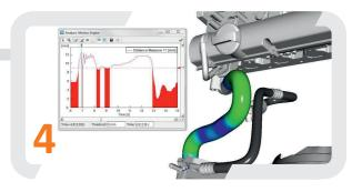
Analyze motions with respect to critical measurements or generate envelopes.
