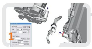
Create cable manually, use the automatic routing or make CAD-geometry flexible easily.
