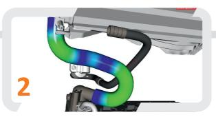
Visualize various analyses like stresses, bending radius, etc. while monitoring critical distances and other measurements.
