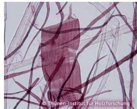
Fiber analysis of a eucalyptus from the Thünen Institute for Wood Research
