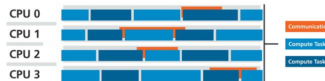
A hybrid-parallel implementation for scalability results in a much better surface to volume ratio and the task based parallelization yields optimal load balancing. The design is multi-threaded with thread-safe matrix assembly and fully threaded matrix finalization.
