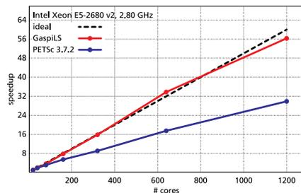
Jacobi preconditioned Richardson, 3D Poisson equation (2<sup>nd</sup> order FD discretization), cubic grid (359<sup>3</sup>)
