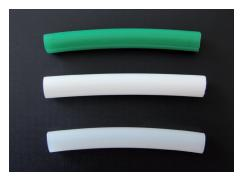
PE tubes with diffusion barriers made of EVOH. The two upper tubes consist of PE-RT, the tube at the botton is made of PE-Xb. The position and thickness of the diffusion barrier can be determined exactly irrespective of the coloring.
