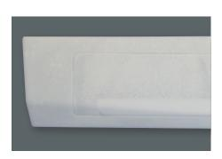
Measurement of airbag cover as an example of engineering plastics: The thicknesses of the predetermined breaking point can be measured
