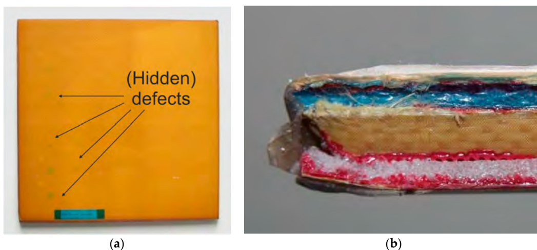
Figure 1. Two photographs of a glass fiber reinforced plastics (GFRP) test sample containing defined integrated defects and features. (a) Top view. Along the left edge of the sample, some of the defects can be recognized shining through the surface layer. (b) Side view. The sample consists of several layers of different materials (e.g., aramid and foams).
