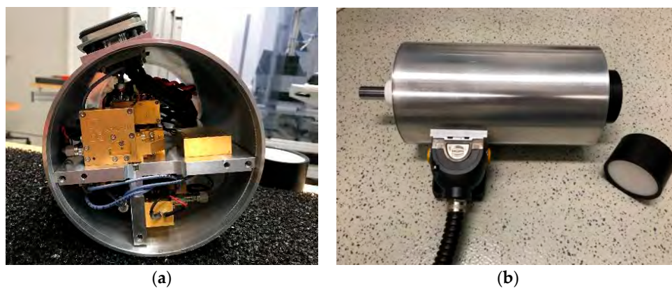
Figure 4. (a) Photograph of the two-frequency sensor head mounted inside a cylindrical metallic housing. (b) Photograph of the assembled measurement device with data I/O and power supply connector. The focusing lens tube can be exchanged depending on the exact measurement geometry and distance of the object under test.
