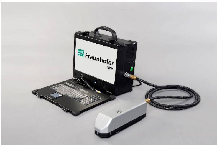
Terahertz-Handscanner © Fraunhofer ITWM
