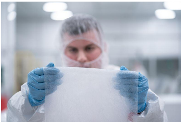
Fig. 1 The nonwovens used for FFP-2 masks must filter at least 94 percent of aerosols, particles or viruses according to DIN.
