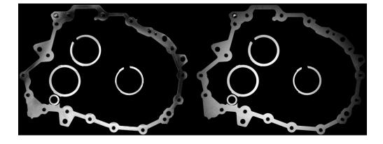
Comparison between a real image from the production line inspection system at the BMW Group (left) and a synthetic image generated using Fraunhofer ITWM technology (right). © Fraunhofer IT
