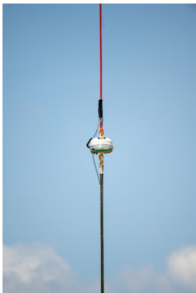
Fig. 2 The CAURUS sensor platform records georeferenced visible and infrared image data during the flight. © CAURUS Technologies
