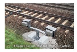
Fault detection during drive-by: Acoustic sensor detects wear condition of axle bearings.
