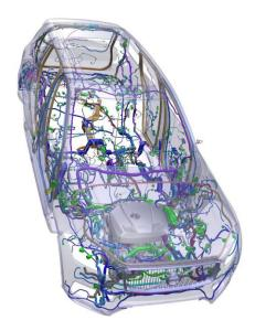
Up to two kilometers of cables are installed in modern cars. © Volvo Cars and Fraunhofer-Chalmers **Research Centre**
