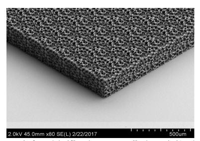
Example of an optimized filter microstructure, a calibration standard 3D-printed by us. © Fraunhofer ITWM
