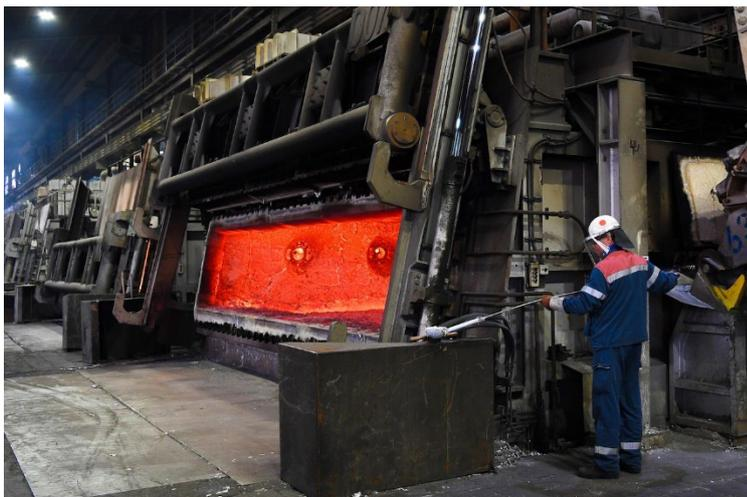
The large melting furnaces of the TRIMET company have an enormous energy consumption.
